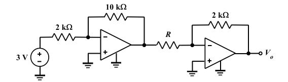
The OpAmps are ideal. Determine the value of *R* required to make  $V_o = 15$  V.
